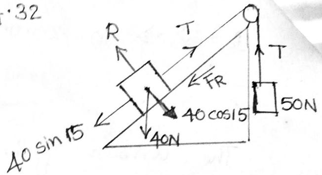
9. Two rough planes inclined at  $30^\circ$  and  $15^\circ$  to the hz. are placed back to back. The masses 15kg and 5kg are placed on the inclined surfaces and connected by a string as shown in figure. If the coefficient of friction is 0.3, Find the resulting acceleration
